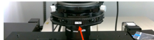
Condenser Prisms- manually controlled by hand
